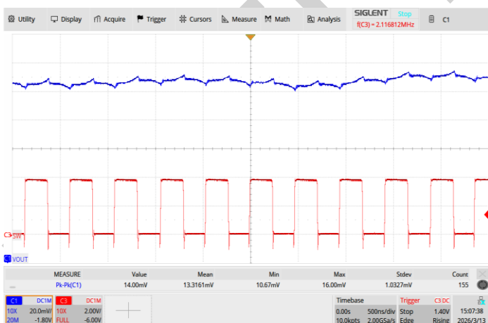
Figure 3-33. V_{out} Ripple, PWM mode, Load =3A
