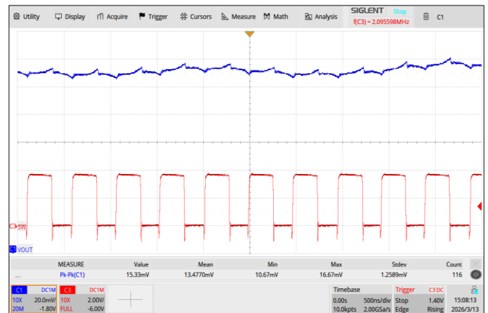
Figure 3-22. V_{out} Ripple, PWM mode Load=3A
