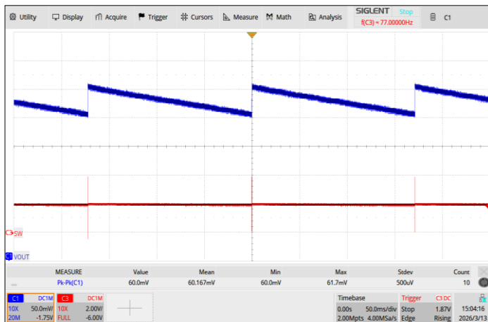
Figure 3-31. V_{out} Ripple, Sleep mode, Load =0A
