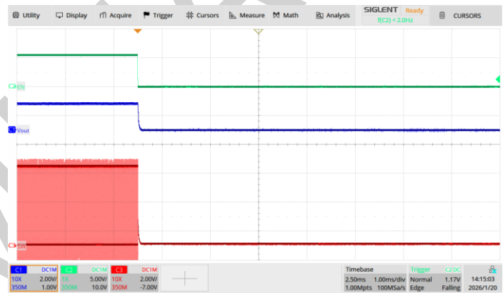
Figure 3-38. Shutdown, V_{IN}=5.5V , Load=2A
