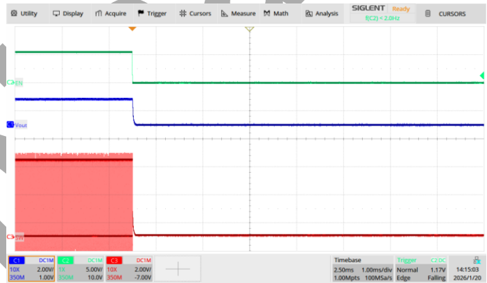
Figure 3-38. Shutdown, V_{IN}=5.5V , Load=2A
