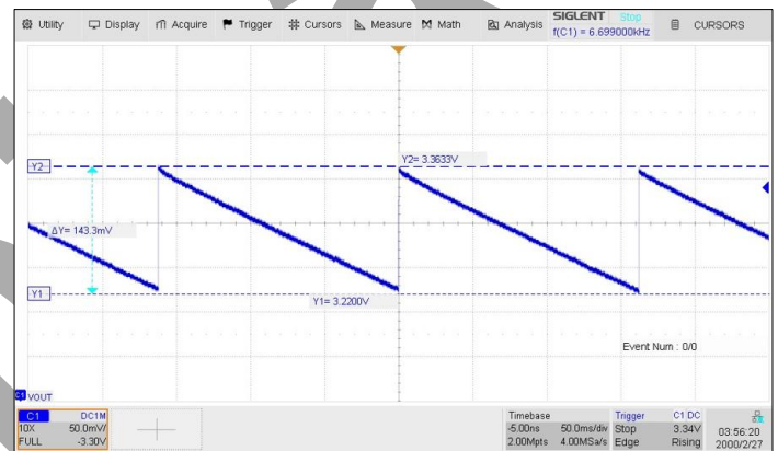
Figure 3-20. Vout Ripple, Sleep mode, Load =0A
