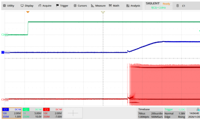
Figure 3-37. Start-up, V_{IN}=5.5V , Load=2A
