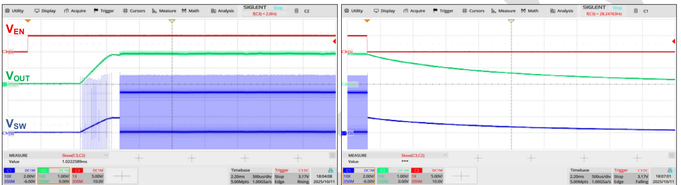
Figure 4-67. Start-up & Shutdown, FPWM Mode, V_{IN} = 5.0V , V_{OUT}=1.8V , F_{SW}=3MHz , I_{OUT}=0A .
